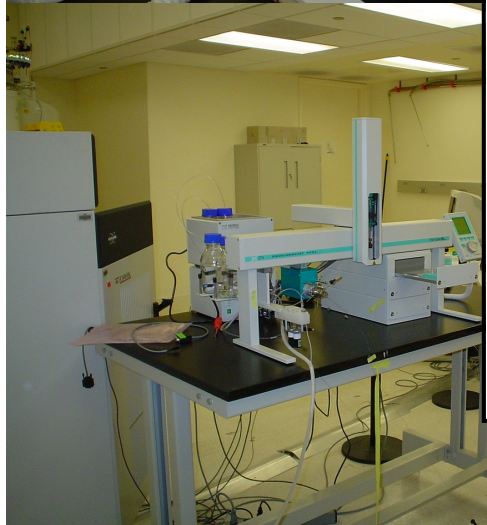
Bruker DPX-400 NMR System with LEAP HTC Liquid Handler, 10µL Sample Volume, 5µL Injection
